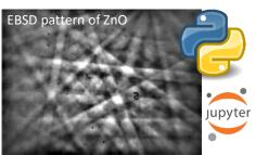
Left: Scheme of EBSD acquisition. Backscattered electrons from a highly tilted sample generate a so-called Kikuchi pattern on a phosphor screen, that is then captured by a camera (<a href="https://en.wikipedia.org/wiki/Electron\_backscatter\_diffraction">https://en.wikipedia.org/wiki/Electron\_backscatter\_diffraction</a>). Right: Exemplary EBSD pattern showing Kikuchi bands from electron diffraction.
